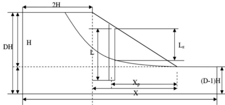
Gambar 2.2 Profil Dari Sistem Stabilitas Tiang (Ho, 2009)
