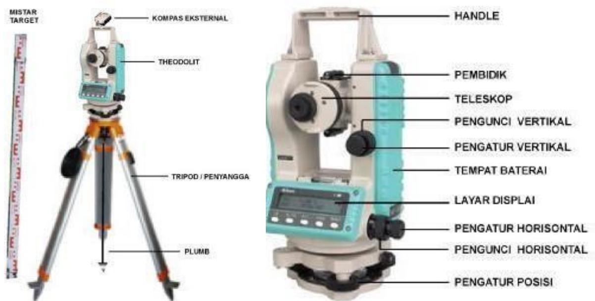
Gambar 2.7 Bagian-bagian Unit Theodolite
